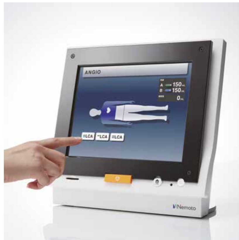
Console with touchscreen operation. Color changes based on mode of operation.
